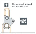
The FRIXION SRB must be correctly orientated with the Attachment Pin/Maillon Cradle at the top and the Sheave at the bottom.
